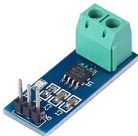
Figure 7. ACS712 Current sensor
