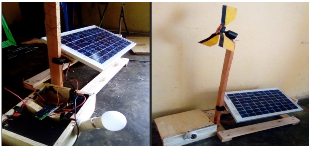
Figure 13. The Hybridized Solar and Wind Renewable Energy Prototype
