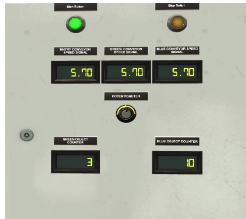
Figure 22. Analog Speed Signal of 5.7 Volts
