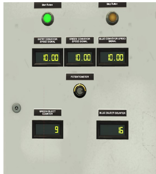
Figure 22. Analog Speed Signal of 10 Volts
