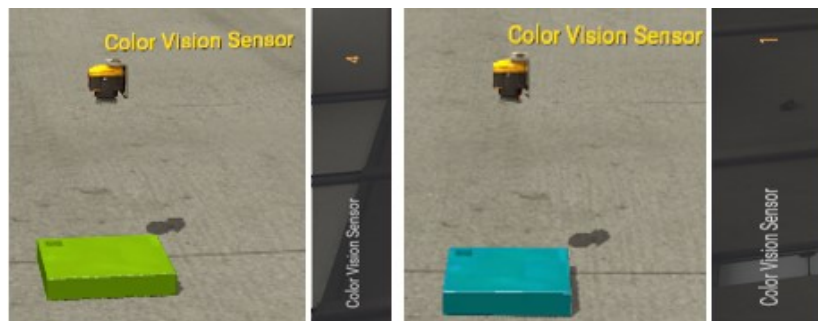
Figure 16. Sensor Returns Value 4 for Green And 1 For Blue Objects
