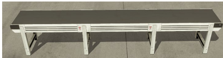
Figure 7. Entry Belt Conveyor
