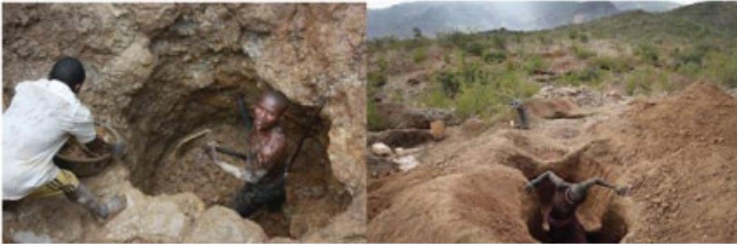
Plate 3: Mine collapses are common place. Such mining pits have high chances of caving in and killing miners.
