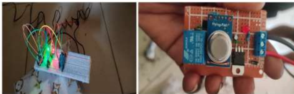
Fig.4: sensor and switching circuit (input devices) prototype
