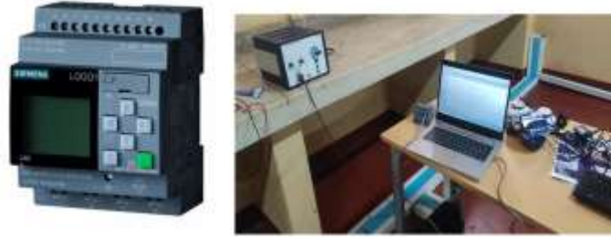
Fig.5: Siemens LOGO PLC and program uploading
