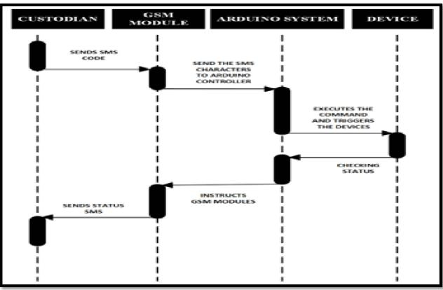
Figure 4: Sequence Diagram of the System
