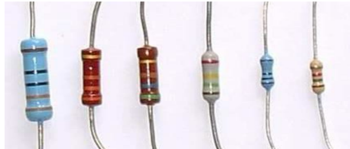
Figure 6. Typical Diagram of Resistors
