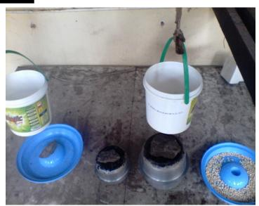
Figure 3: Part of experiment set up without cupboard storage. Hanging buckets representing hanging baskets storage, modified saucepans (Metallic container) to illustrate metallic drum storage and exposed seeds as control set up.
